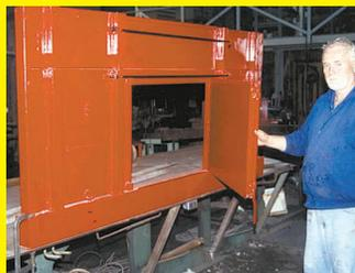
one didn't let the grain flow out fast enough. The new door lets grain flow 1 1/2 times faster. I also put the door latch low so anyone can open it. If I wanted to, I could cut a slide in it to insert an auger. **(Clair Wilson, Winchester, Ill.)**
