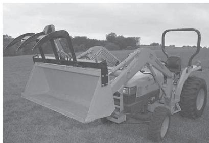
Grapple fork fits compact tractors with a 5 or 6-ft. wide bucket. It comes with a telescoping mounting frame that attaches to each side of the bucket. The frame is designed to accept either single or double grapples. A single grapple sells for \$500; a double for \$850.
