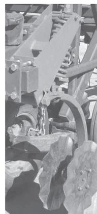
"It works on any brand of chisel plow and in some cases may save you the cost of buying a new stalk chopper," says Ron Tschetter. The kit for each shank consists of two 18 or 20-in. dia. waffle coulters and the mounting hardware needed to bolt them onto the shank.
