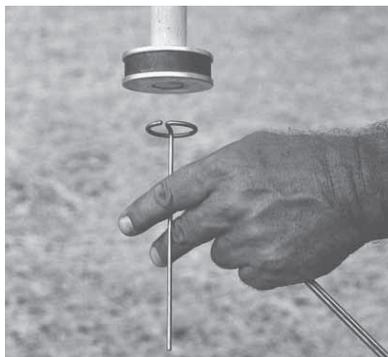
"Pounder" is a lightweight wooden rod with a round magnet at the bottom. It punches through the mat into the ground. The pins disintegrate in 1 1/2 to 2 years.
