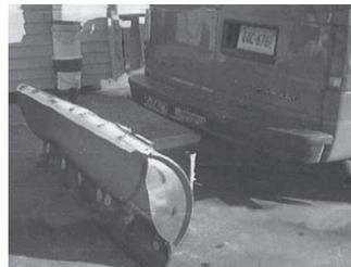
"The right side of the blade is even with the van. The left side sticks out to the side a little, so as I back up I can look in the driver's rear view mirror and see the snow flying out. The right side of the blade makes a nice clean cut out against the curb or driveway," says Brian Hoadley.
