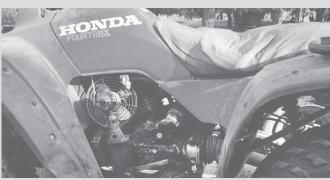
"It lets me operate the ATV at idle all day long without ever overheating the engine," says Doug Fluit. "I've put hundreds of hours on my ATV since I added the fan, with no problems. I think the same idea could be used on any ATV equipped with a 12-volt hattery."
