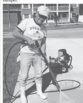
"I use a Honda 3,400-lb, psi pressure washer around my home to clean my driveway, etc. With that much pressure the wand is always exerting an upward pressure on my arms, which really gets tiring. To counterbalance the upward pressure, I added a 2-ft. length of 5/8-in. thick rebar to the wand, securing the rebar to the wand with plastic wire tires. Now the wand actually floats, and all I have to do is guide it. I've used this idea for several years and it works great."
