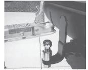
I accidentally overshot the ball hitch on back of the car and the trailer's tongue just nicked the car's plastic bumper. Luckily, the impact didn't crack the bumper. To prevent that accident from ever happening again, I welded a 6-in, long by 3-in, wide, 3/8-in, thick steel plate to the top of the hitch. Now if I ever overshoot the ball, the steel plate will keep the trailer tongue from ever hitting the bumper.
