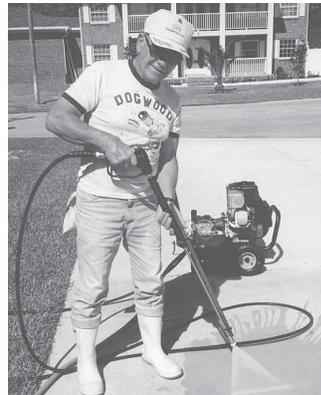
"I use a Honda 3,400-lb. psi pressure washer around my home to clean my driveway, etc. With that much pressure the wand is always exerting an upward pressure on my arms, which really gets tiring. To counterbalance the upward pressure, I added a 2-ft. length of 5/8-in. thick rebar to the wand, securing the rebar to the wand with plastic wire ties. Now the wand actually floats, and all I have to do is guide it. I've used this idea for
