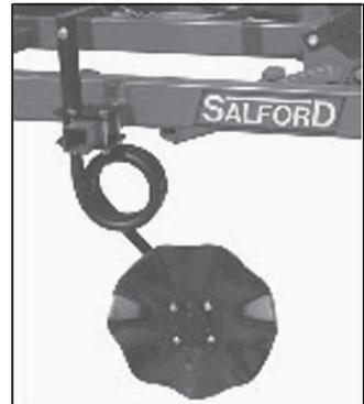
Individually-mounted spring coulters are designed with a 1 1/8-in. wound coil to keep from pulling up stones.
