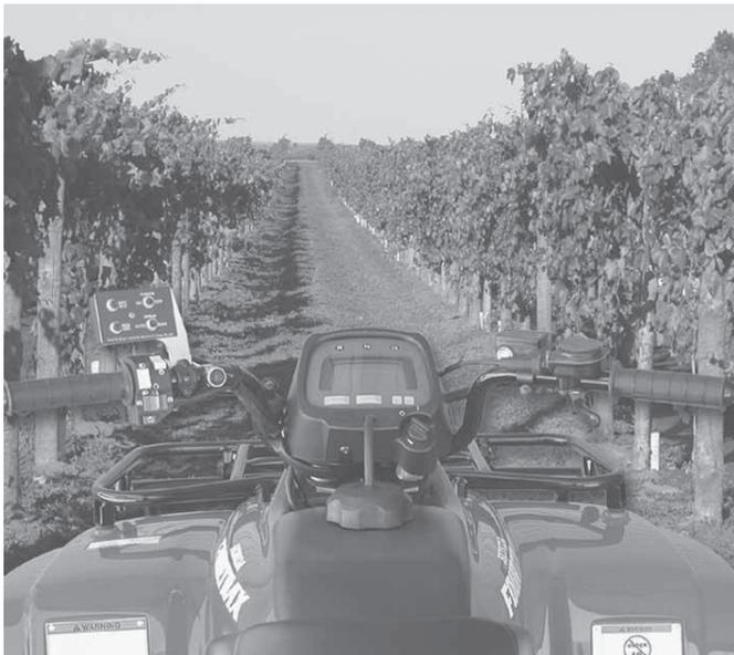
QuadCruise cruise control lets you set a constant speed from 2 to 15 mph. It's especially valuable when spraying or applying fertilizer, says the manufacturer.
