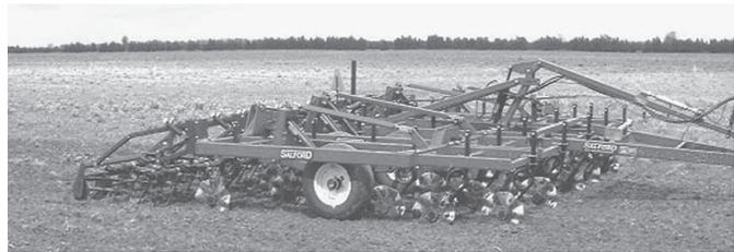
Residue Tillage Specialist (RTS) has 5 to 6 ranks of wavy residue coulters on front and standard harrows at the back, which spread residue and level the field.
