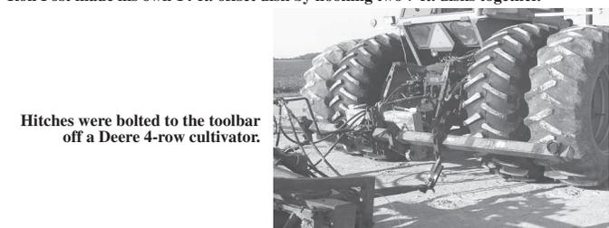
Hitches were bolted to the toolbar off a Deere 4-row cultivator.
