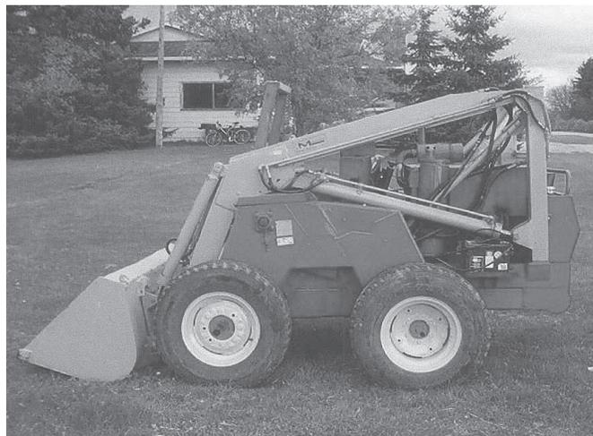
Bill Bell used scavenged parts from three self-propelled swathers to build this skid steer loader. It's equipped with a 6-ft. Deere loader bucket.
