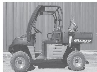
Aftermarket lift kit raises the vehicle suspension, boosting ground clearance and providing room for bigger tires.
