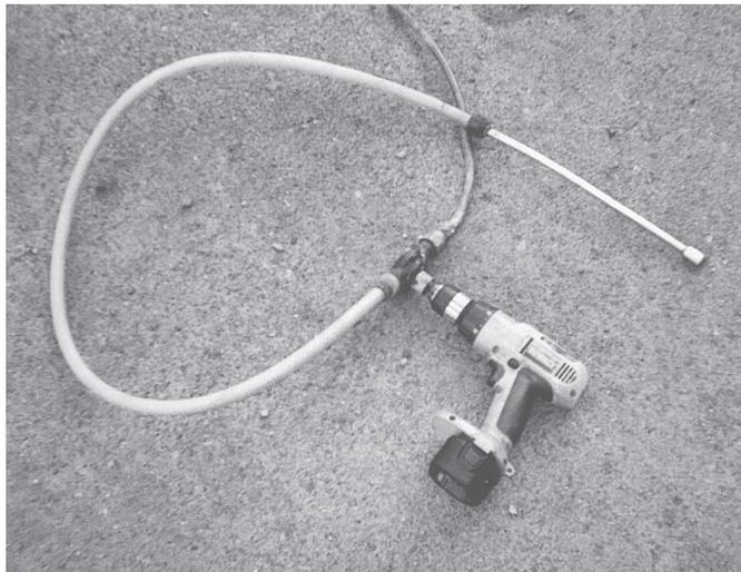
Cordless drill shaft-drives a small pump. Pump has a 5-ft. long plastic hose attached to one side and a copper suction line to the other.
