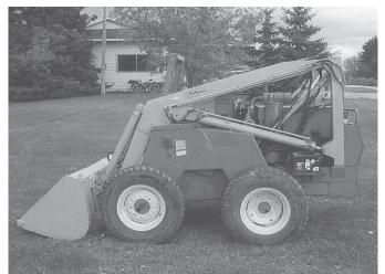
Bill Bell used scavenged parts from three self-propelled swathers to build this skid steer loader. It's equipped with a 6-ft. Deere loader bucket.
