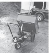
Home-built wheelbarrow is powered by a 6 1/2 hp garden tractor engine and hydro-static drive unit. The 48 by 30 by 15-in. deep box is balanced for easy dumping. Contact: FARM SHOW Followup, Daniel 13778 (ph 607 656-8322; djkirkjr
