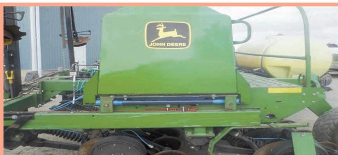
Load bars under seed box are visible from end of drill.
