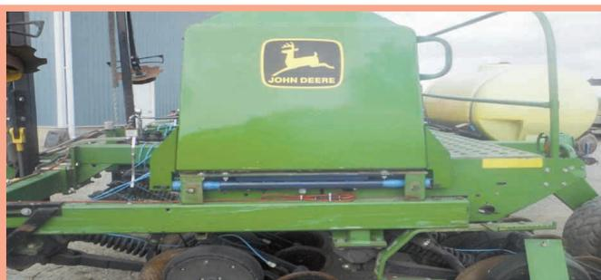
Load bars under seed box are visible from end of drill.
