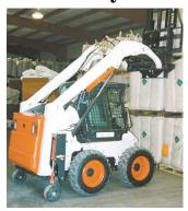
Kit consists of a pair of 4-in. wide, 10-in. high caster wheels that bolt onto side of skid loader, just behind the rear wheels.
