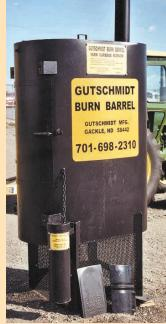
Garbage burner is made from an old fuel oil tank and has an enclosed design for safe burning. It drafts from the bottom for a fast burn
