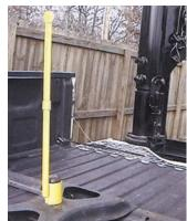
Upright poly pole fits over hitch ball. As you back up you line up the gooseneck until it just touches the hitch guide. Then you remove the hitch guide and lower the gooseneck onto the ball.
