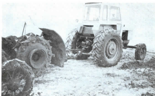
The "Rotovator" consists of two 5-ft. dia. steel discs mounted together on truck rims.
