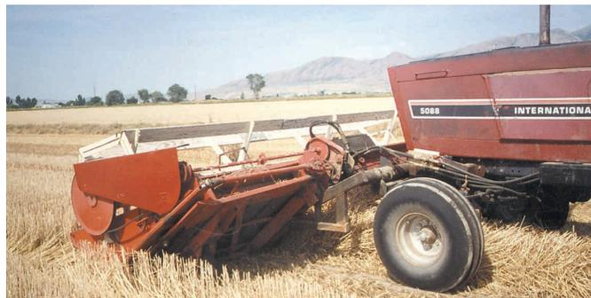
Hege bought a used header and had a local welding shop fabricate brackets for his Case IH 5088 tractor.
