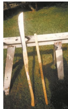
Chopper was made by attaching a machete blade to the end of a 28-in. axe handle
