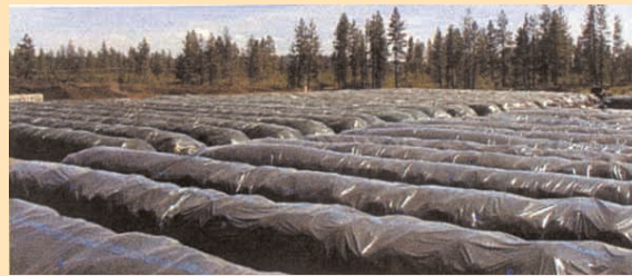
A 200-ft. long, 5-ft. dia. "EcoPOD" bag holds about 76 tons of material or 250 cu. yds.
