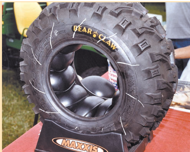
Rubber “air balls” inflate to 4 to 30 lbs. of pressure and are squeezed tight inside tire. Each air ball has its own valve.
