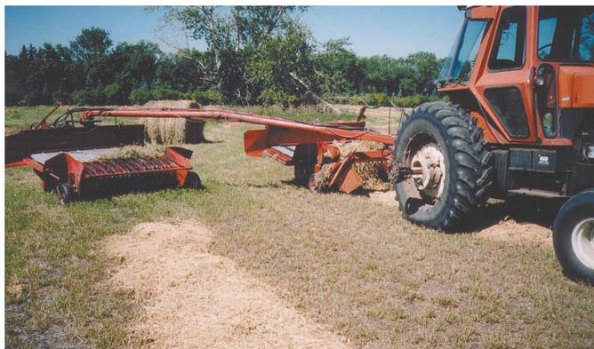
Swath turner consists of two home-built swath turners hooked in tandem on a hydra swing tongue.
