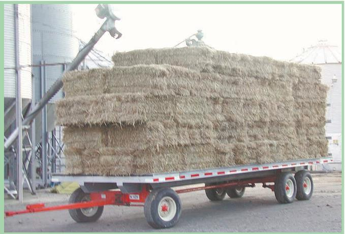
Beds are available in lengths from 14 to 30 ft. A 25-ft. bed can haul up to 315 32-in. small bales at a time.
