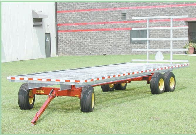
All-steel wagon bed comes with an expanded metal grating floor, stake pockets, and removable back panel. If you want you can mount it on your own running gear.
