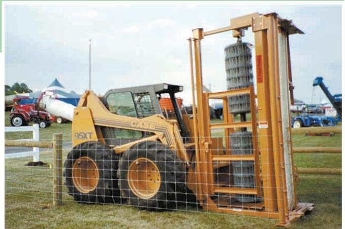
“Easy Fencer” is designed to fit any skid steer loader and can unroll up to six wire strands at a time.
