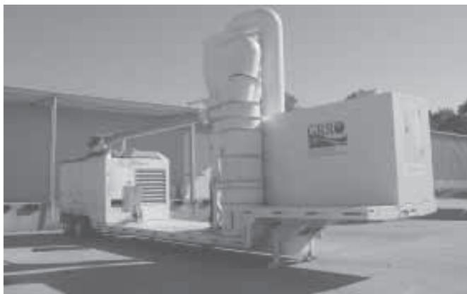
"We can take just about any waste stream and dry it down into compost-type fertilizer that's ready to bag," says Loran Balvanz about the new Tempest Air Drying System.
