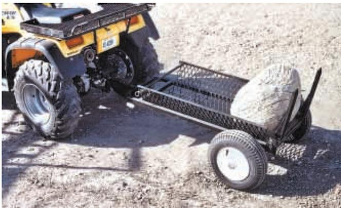
ATV towable hand cart has a hitch on top that hooks up to the ATV drawbar, and a pair of adjustable prongs to load rocks.
