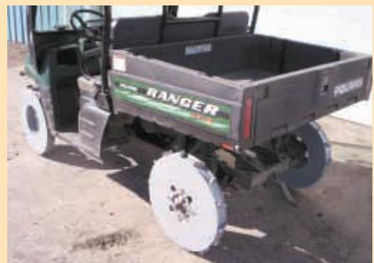
Raguse also offers new 3-in. wide wheels that are designed for heavy truck-type ATV's. Wheels are built to handle power spinning by an ATV's rear wheels while trenching.
