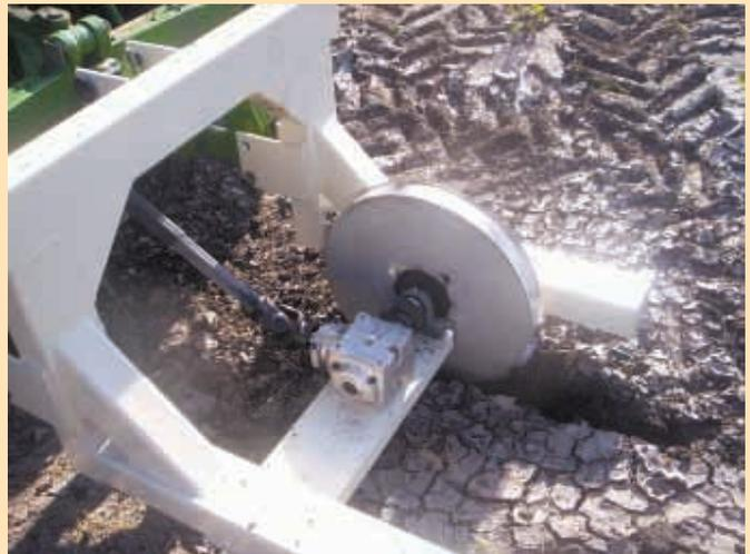
Tractor pto drives a 90 degree gearbox that's attached to wheel.
