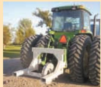
Power trencher wheel is 3 in. wide at the outer edge and has 1-in. angled lugs.
