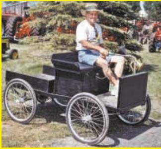
of plywood over a frame made from 1 by 2-in. rectangular tubing. The vehicle has tiller steering and a squeeze bulb horn on front, and a small wooden box on back. The vehicle's 8 hp Briggs & Stratton engine and 5-speed transmission are out of a 1968 Deere riding mower.
