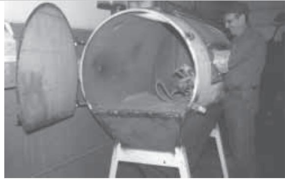
Litchfield cut out one end of tank to make an access door and cut off the bottom of the tank to weld in a home-built metal hopper.
