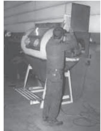
Tank has an air-powered blast gun that's pre-plumbed into a quick-tach air hose.
