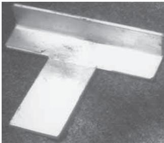
**Leonard Seltzer, Manhattan, Ill. ph 815 478-3578:** "I came up with a simple T-shaped metal bracket made from 1 1/2-in. angle iron and flat steel plate that makes it easy to weld two pipes together at a 90 degree angle. It keeps the pipes from rolling around and getting off center."
