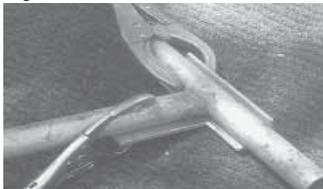
"The bracket measures about 8 in. long by 5 in. wide. I use a small square to line up the pipes and a pair of vise grips to secure the pipes to the bracket."
