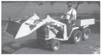
Connecting the two axles was a tricky job. To match up the frames, Brown had to turn the add-on frame upside down, reversing the position of the two halves of the frame.
