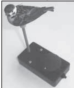
The decoy emits a constantly changing sequence of chirps while it is moved around by a small electric motor.
