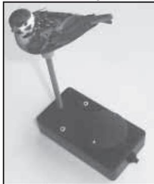
The decoy emits a constantly changing sequence of chirps while it is moved around by a small electric motor.
