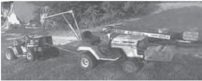
Doug Brown bolted part of the frame off an old riding mower on front of the tractor to hold concrete blocks for weight. On back, he added a hand pump hydraulic lift off an old handicap lift.
