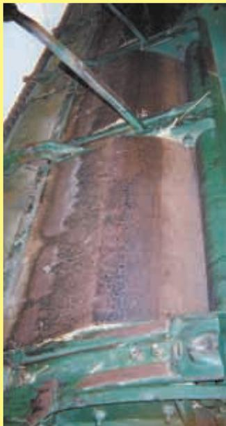
**Heavy steel skid plates are installed behind existing poly skid plates that are standard on many grain headers.**
