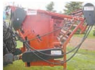
**BeddingPro bale shredder attaches to a 3-pt. hitch or quick-tatches to a front-end loader. It shreds and fluffs straw so well livestock producers can extend bedding intervals, says manufacturer Paul Fox.**
