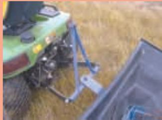
Ehrman also made hitch on tractor. Auger hitch fits over fixed pin on drawbar.
