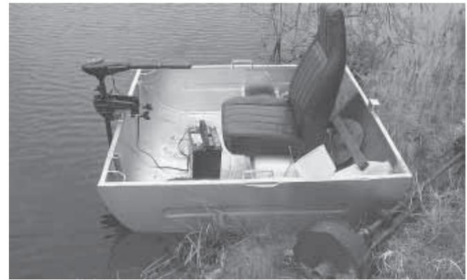
"Once I get the boat in the water, I just take the transport wheel off and throw it behind a seat," says Leroy Groening. Boat measures 4 1/2 ft. wide by 5 ft. long. When done fishing, Groening attaches the wheel next to the motor and rolls the boat up a plank into his pickup bed.
