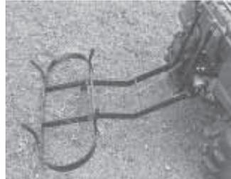
Oval-shaped lift frame pivots on bracket at back of ATV. It’s raised up by an electric winch that operates off ATV battery.
