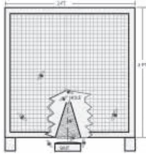
Fly trap consists of a 2-ft. sq. wood cube covered with window screen. A 4-in. dia. inverted cone is set in bottom. Flies go up cone and can’t figure out how to get out.
