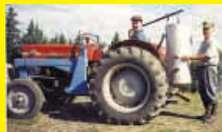
This photo shows my son Bradford and I with a one-row, 3-pt. mounted granular fertilizer spreader we made out of an old 30-gal. hot water heater. We use it to fertilize potatoes about one week before cultivation.
