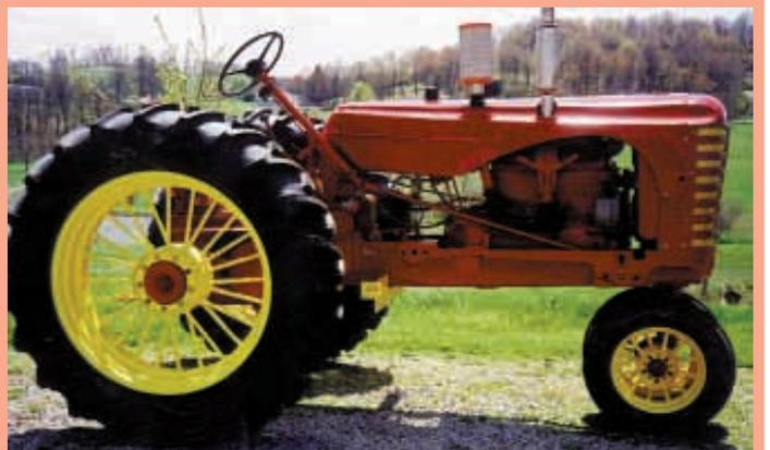
I'm sending along a photo of my antique Massey Harris 444 tractor and the home-made spoke wheels I built for it. The spokes are made out of 3/4-in. dia. steel and are welded to wheel rims that measure 11 by 38 on back and 16 in. on front. To hold everything in place, I fabricated a jig out of 6-in. channel iron in the shape
