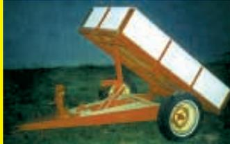
in. sq. tubing that came from an old piece of machinery. It's covered by 1/2-in. thick plywood. The bed has 1-in. wide, 8-in. high plastic sides that came from our father's hay barn. The cart is equipped with a winch and cable hoist that allows it to dump 2,000 lbs. or more. We use the trailer to haul grass, straw bales, dirt, rocks, and so on. Our family loves this cart because it's easy for everyone to use. (Darin Van Well, 30637 131st St., Selby, S. Dak. 57472 ph 605 649-1288)
