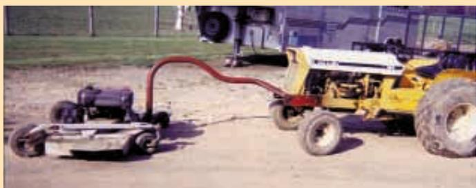
Thank you for the story on my gooseneck-mounted mower deck (Vol. 26, No. 3). It consists of a 60-in. mower deck that I mounted on front of my 1981 Cub Lo Boy tractor. Works great for mowing fence corners and ditches and also eliminates a lot of hand trimming around trees and buildings. The front of the deck is equipped with a home-built gooseneck ball hitch that allows the mower to swivel 360 degrees when turning or backing up.
