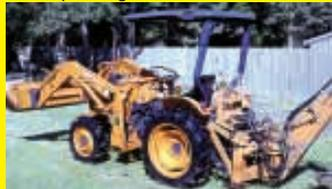
protection bar. I even mounted a 12-volt fan under the canopy in the back for ventilation during hot weather. I painted the canopy Kubota blue. It keeps both the sun and rain off me. (Terry and Debbie Benoit, 1077 Bobcat Road, Orange, Texas 77632)
