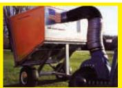
A 3-pt. mounted, pto-driven blower sucks leaves up and blows them into the box. The top of the box is made from perforated metal which serves as an outlet vent. All the grass clippings and leaves empty out when the unit is fully raised.
