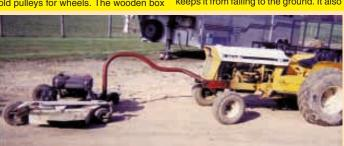
Thank you for the story on my gooseneck-mounted mower deck (Vol. 26, No. 3). It consists of a 60-in. mower deck that I mounted on front of my 1981 Cub Lo Boy tractor. Works great for mowing fence corners and ditches and also eliminates a lot of hand trimming around trees and buildings. The front of the deck is equipped with a home-built gooseneck ball hitch that allows the mower to swivel 360 degrees when turning or backing up. I'm sending better photos of the unit.
