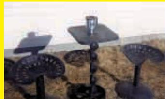
between the seats is supported by a length of auger flighting, which I welded to an old cast iron pulley that serves as a base. (Pete Peters, Box 166, Osler, Sask., Canada S0K 3A0 ph 306 239-2045)
