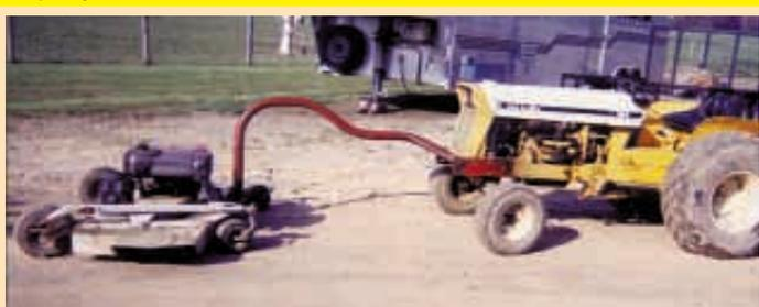
Thank you for the story on my gooseneck-mounted mower deck (Vol. 26, No. 3). It consists of a 60-in. mower deck that I mounted on front of my 1981 Cub Lo Boy tractor. Works great for mowing fence corners and ditches and also eliminates a lot of hand trimming around trees and buildings. The front of the deck is equipped with a home-built gooseneck ball hitch that allows the mower to swivel 360 degrees when turning or backing up.
