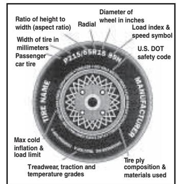
ber, the greater the load carrying capacity of the tire. The letter is the speed rating, based on indoor wheel tests and doesn't represent a safe or acceptable driving speed.
