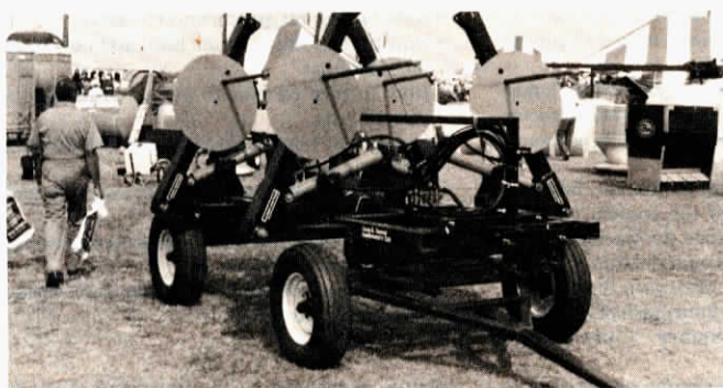
Bale hauler has two spikes on either side and one at rear (not visible in photo).
