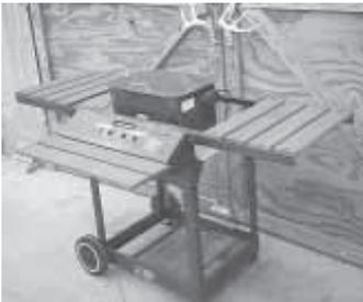
"I also converted an old gas grill that didn't work any more into a portable parts washer, by replacing the grill with a 3-gal. electric-operated parts washer. I use the grill's folding front and end sections to hold parts. The
