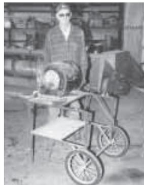
**Art Leefers, Carlinville, Ill.:** Art never sweats when working in his shop or around the yard on a hot summer day thanks to his portable high-volume fan, which was built for him by a friend, Dale Johnson. A squirrel-cage fan out of a junked furnace mounts on the frame of a cart fitted with high wheels and stationary front legs. The big wheels make it easy to move around.
