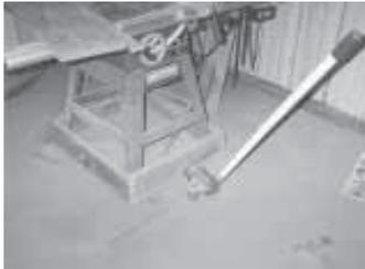
use them to move my table saw around my shop. Two wheels and their adjoining support brackets are permanently bolted to a square wooden base that's bolted to the bottom part of the table saw's legs. A small steel ring is bolted to the front side of the base.
