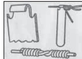
"The other drawing shows the splicer in position on the wire. The splicer should be turned backward, as shown in the drawing, to make the splice. A pair of large pliers should be used to hold the two wires between the coils while turning the splicer."
