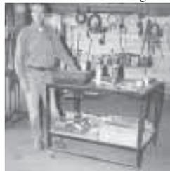
steel tubing and measures 3 ft. wide and 5 ft. long. I'm 6 ft. 3 in. tall so I made the unit higher than most commercial shop tables. It has a plywood top that's about waist high so I don't have to bend over. There's also a plywood shelf down below. The table really comes in handy for working on objects such as small engines, etc. I can roll the table close to the tools I need to use."
