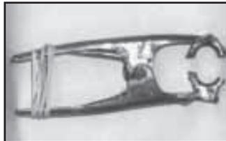
solve the problem I found a nut that would fit the adjustment bolt and welded it between the jaws of a spring clamp. Then I sawed the nut in half. To adjust the depth stop I just lower the spindle on the drill press and slip the nut in place onto the adjusting bolt. It eliminates the need to run the nut up or down the adjusting bolt.
