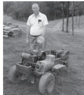
removed the rear deck and axles and created a hitch point to allow the unit to be towed around. On the former front end I welded the steering mechanism to make it trail straight. The generator was rigged to take its power from the front of the engine. There's an electric clutch on the engine pulley. I used a 5,000-watt generator. I rigged the electrical system to where a single plug-in can run the power for all my needs."
