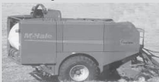
60 wrapped bales per hour in a heavy crop. The machine features a single control box that monitors and controls all operations. It even features an auto greasing system that automatically feeds a small bit of grease to bale rollers after each
