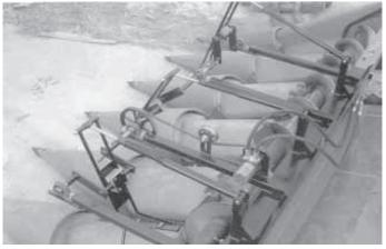
Header sweep assembly is powered by a hydraulic motor that attaches to combine's reel drive. It has fingers that straddle the center three snouts in a row crop header.
