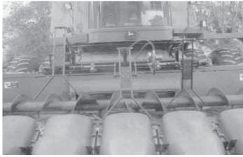
Fingers pull material up the snouts toward the auger, then raise up, extend forward, and then drop down again over the snouts and repeat the action.
