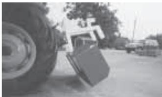
Bucket is equipped with 3-pt. brackets on front and back so it can be reversed, allowing you to use it in either direction.
