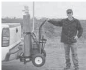
**Two-wheeled cart mounts on receiver hitch, making it easy to transport without having to lift it into pickup.**
