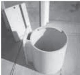
**Post puller consists of two parts - a steel saddle that welds onto side of bucket, and a 10-in. dia. steel pipe that slips into saddle and locks in place with one pin.**
