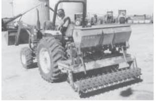
The 5-ft. wide seeder is fitted with a pair of 8-in. dia. aerating rollers. Grass seed hopper drops seed onto ground between rollers.
