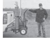
Two-wheeled cart mounts on receiver hitch, making it easy to transport without having to lift it into pickup.
