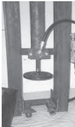
Round pusher plate attaches to end of hydraulic cylinder.
