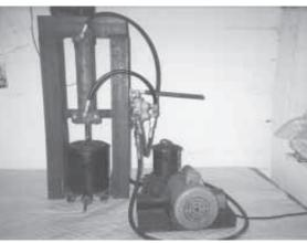
Frey's 2-gal. capacity sausage stuffer is operated by the power steering pump from an old truck. A hydraulic cylinder is attached to a plate that pushes meat through stuffer to fill sausage sleeves.
