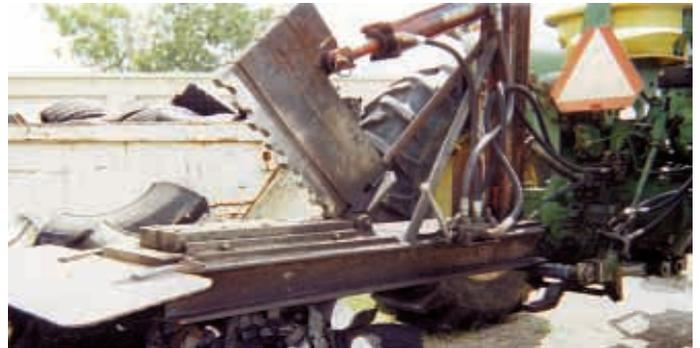
Ray Mickan's home-built tire cutter mounts on a tractor 3-pt. hitch and uses a hydraulically-powered knife to cut through tires.
